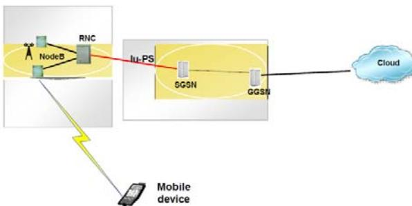
Fig. 3. Mobile device communicate with Cloud through WCDMA [5]
